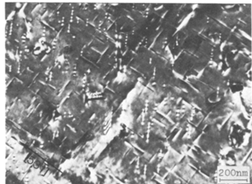
Figure 6 GP zones situated in three mutually perpendicular directions, observed in foil aged for 2.16 \times 10^4 sec at 463 K.
