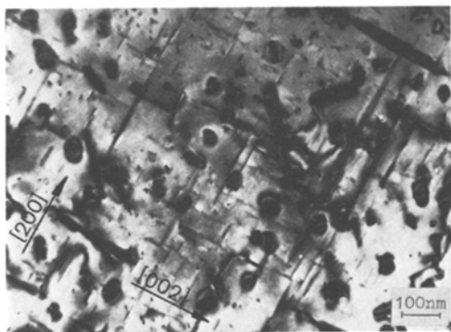
Figure 7 Rod-like \beta' precipitates in Al-9 wt% Si silumin, lying in \langle 010 \rangle directions.
